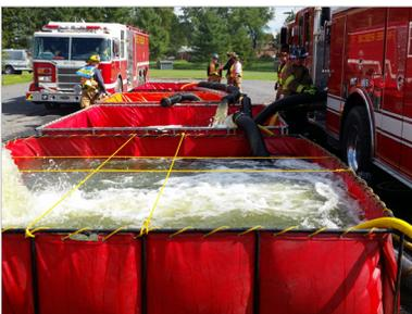
FOL-DA-TANK folding frame portable water tanks are designed for rural areas where water is difficult to supply. FOL-DA-TANK collapsible tanks double the firefighting capability at the fire scene.
